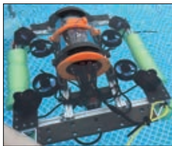
The autonomous robotic submarine, Orange, designed and built by Team Inspiration. (photo by Teresa To)
