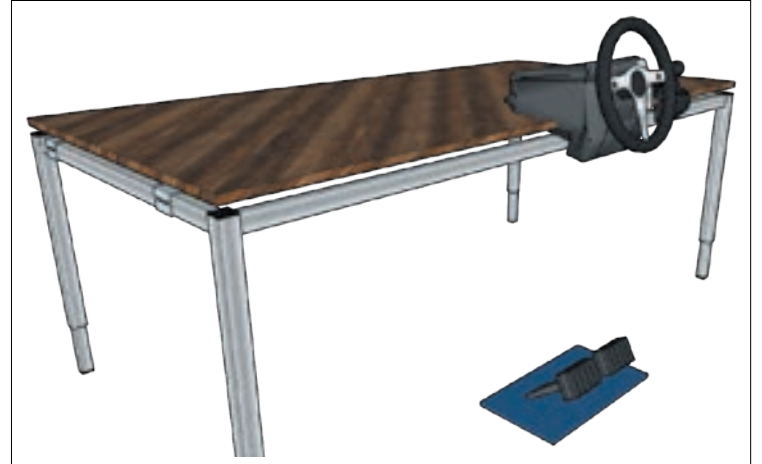
Rendering of hardware components for the VirtuRoad virtual reality driving simulator. (courtesy image)
